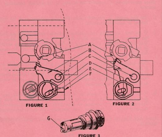
Plate B is pivoted at point C and moves from the position in Figure 1 to the position in Figure 2 by the action of the lock cylinder explained later. Plate A, which is in effect a ratchet, is rotated by the square shank of the door handle when opening and closing the door. When plate B is engaged with ratchet plate A as in Figure 2, the mechanism is locked and the door handle cannot be turned.
